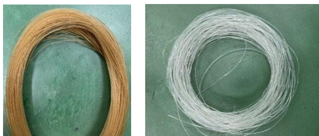
Fig. 1 (a) Kenaf fibre PLA composites filament (b) Neat polymer filament
