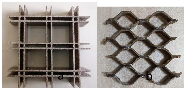
Fig. 1: Photograph of (a) square interlocking core and (b) honeycomb core of flax/PLA
