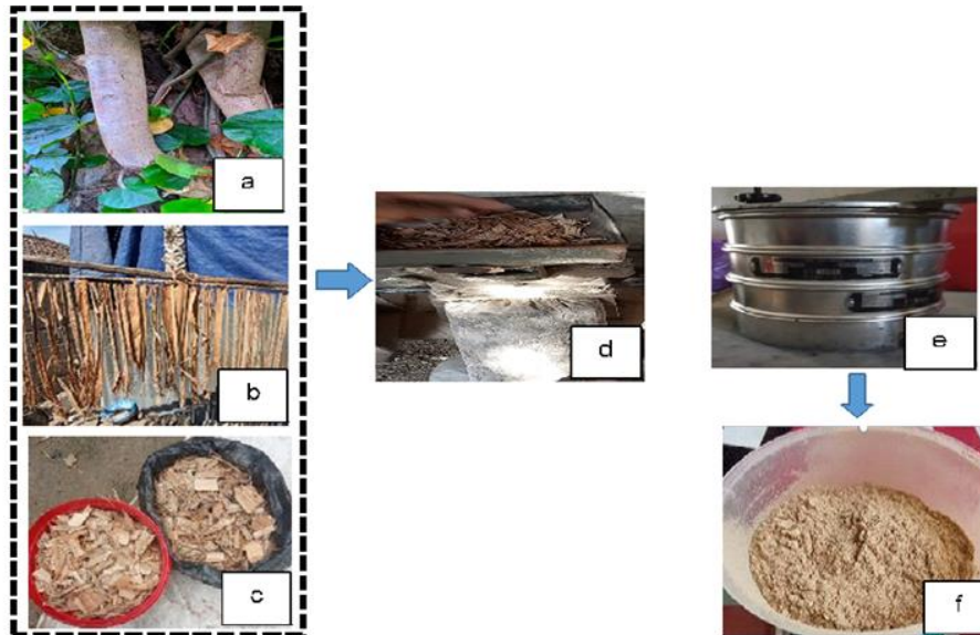
Fig. 1 Process of making powder, (a) HT branches, (b) HT fibers, (c) shredded of fibers, (d) fiber milling, (e) fiber sieving, (f) hibiscus tiliaceus powder (PS).
