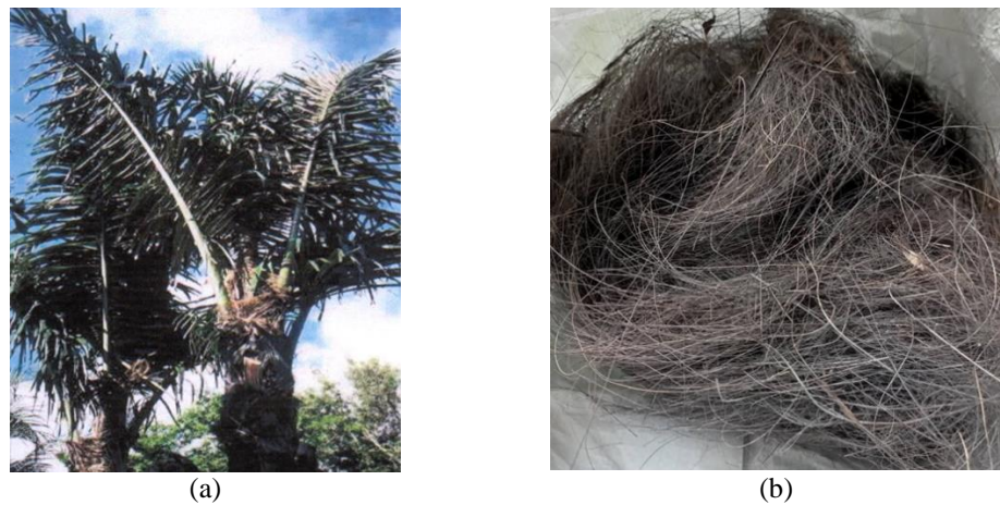
Figure 1. (a) Sugar palm tree and (b) its black fibre or widely called as sugar palm fibre, obtained from Kuala Jempol, Negeri Sembilan, Malaysia
