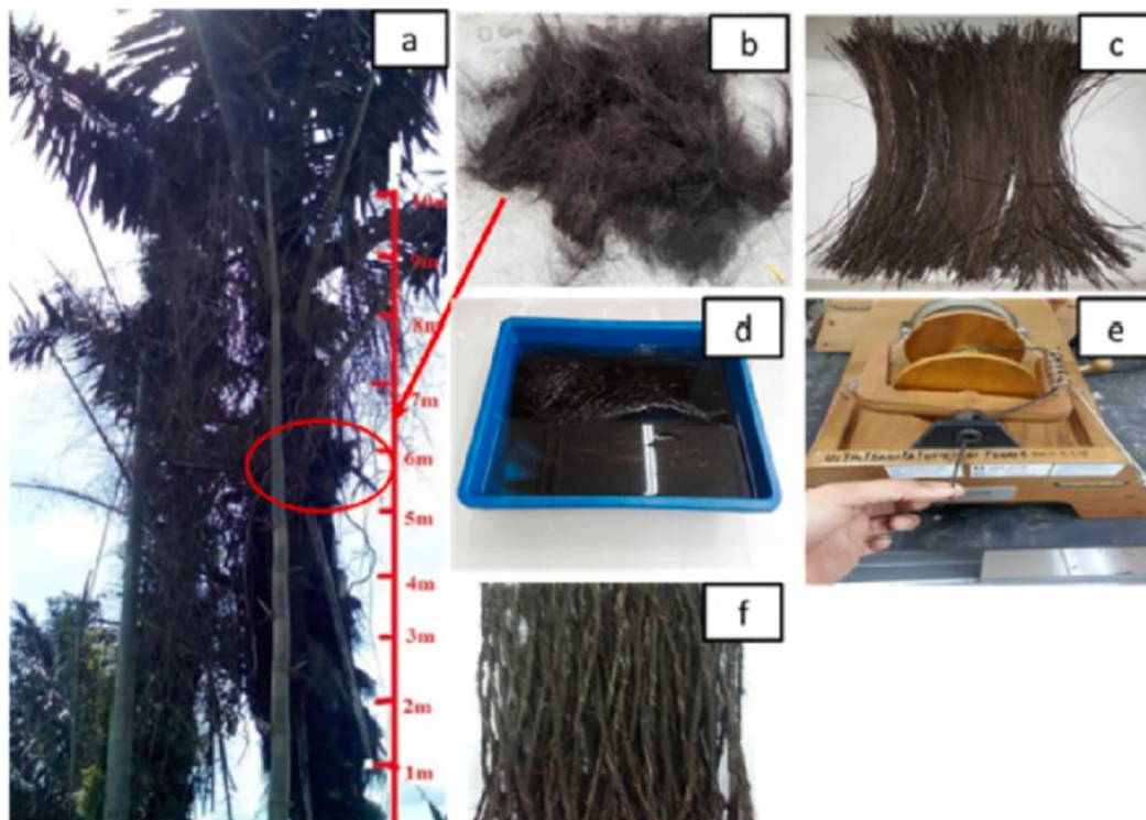
Figure 1. Preparation of SPF from sugar palm tree: (a) locating suitable SPF at the trunk, (b) SPF bundle, (c) combed SPF, (d) SPF treatment by alkalisation, (e) fibre yarning, and (f) finalised SPF yarn. Adapted with permission from Ref. [85]. Copyright Elsevier
